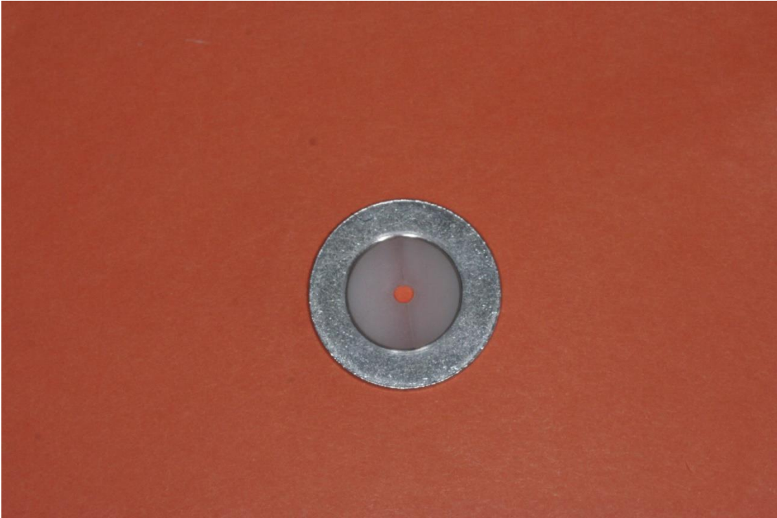
Figure2 The special mold (3 mm × 3 mm).
