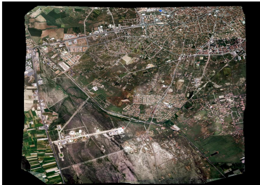
Figure 6. The Orthophoto Mosaic Image For The 25 cm Ground Sample Distance.
